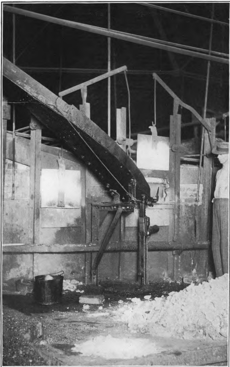
PLATE 11.—A SOFTENING FURNACE IN REFINERY, WITH MECHANICAL CHARGING.
